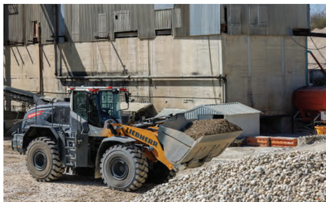
Liebherr's autonomous wheel loader carries out the job completely independently in a defined work area and continuously adapts to a changing environment.
