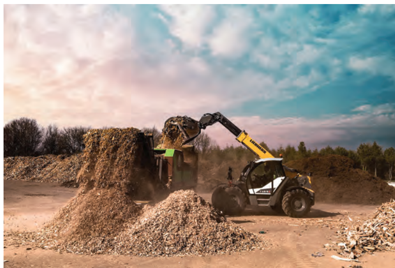
ABOVE: The new T 48-8s telehandler marks Liebherr's entry into the 8-m lift-height class and represents a strategic extension of the range in the industrial segment.
