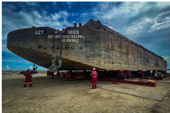
Setting down the barge onto climbing jacks at the launching site.
