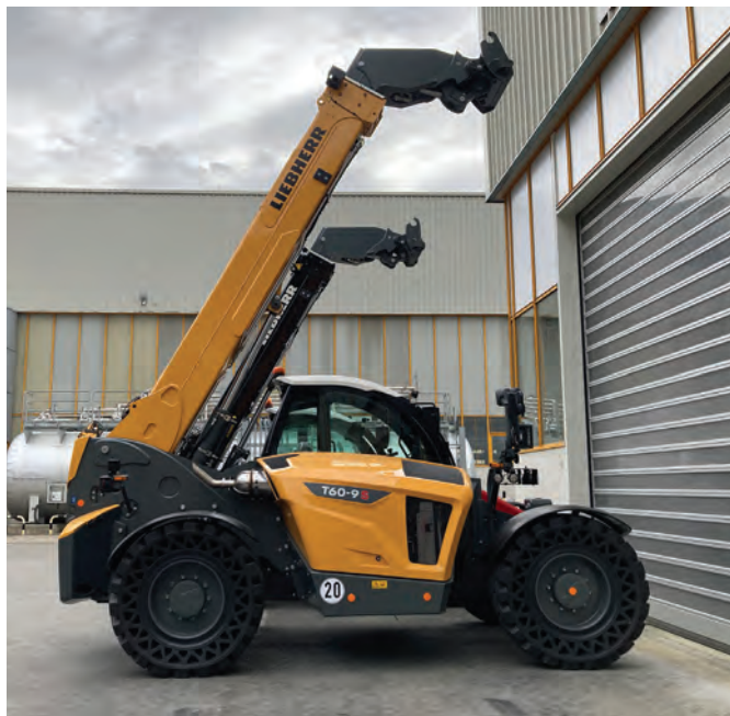
ABOVE AND LEFT: The Generation 6 telehandlers, seen here in Telfs, are available to global markets and suitable for a wide range of industries. Load capacities of up to 4.2 t in the 'S' models have been increased by up to 9% compared with their predecessors.
