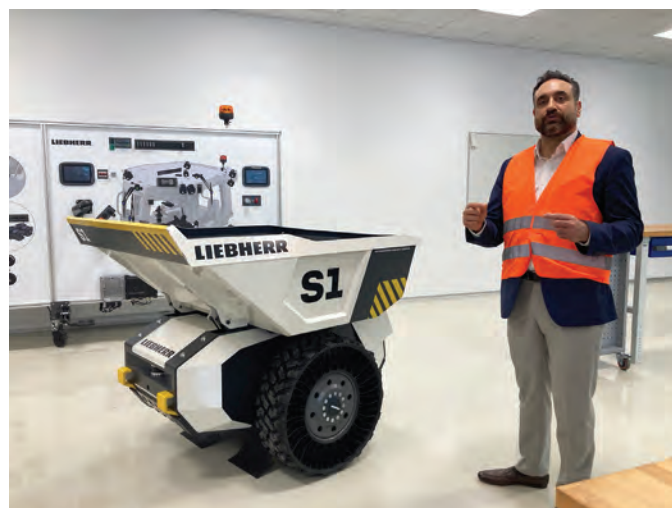
BELOW: Altan Enginlev, CEO of S1 Vision, presents the new haulage concept to the media. The truck is scalable, offering a payload ranging from 220 kg up to 131 t.
