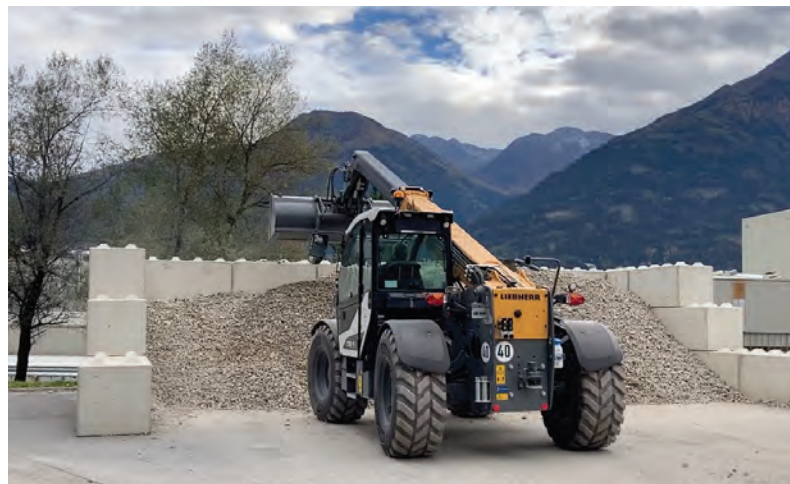
ABOVE AND LEFT: The Generation 6 telehandlers, seen here in Telfs, are available to global markets and suitable for a wide range of industries. Load capacities of up to 4.2 t in the 'S' models have been increased by up to 9% compared with their predecessors.
