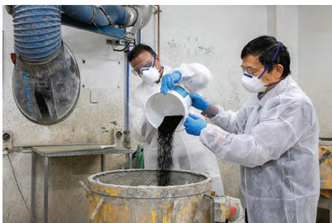
Dr Rajeev Roychand (left) and Professor Jie Li add coffee biochar into a concrete mixer in their lab at RMIT University.
