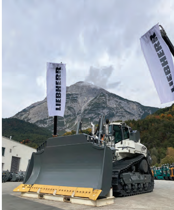
The PR 776 G8 dozer on display at the Telfs facility. Delivering 565 kW, the machine is designed for the most challenging heavy-duty tasks.
