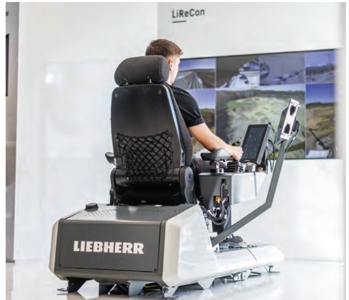
With LiReCon system, Liebherr machines can be controlled remotely via the real operator workstation, equipped with all the necessary controls and system information.
