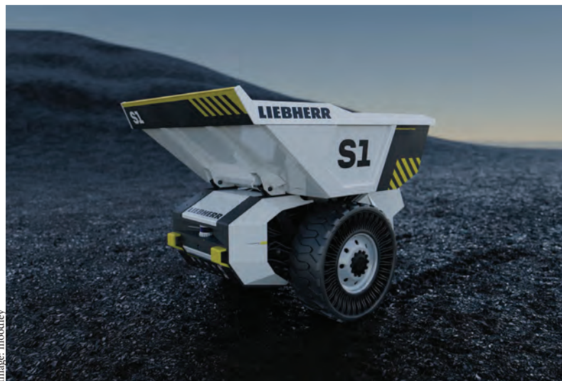
ABOVE: The S1 Vision haulage concept is designed to focus on the core components necessary for moving material. It features a self-levelling system to ensure maximum stability and safety, even on bumpy or rough terrain.
