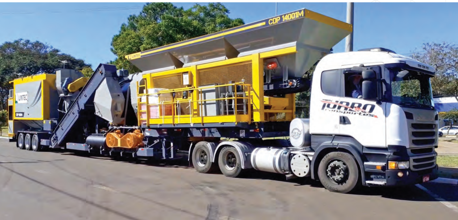
The mobile Lintec CDP1400M asphalt mixing plant supports Mexico's road modernisation programme. The unit features high-output performance with up to 15% RAP for greener, more cost-effective construction.
