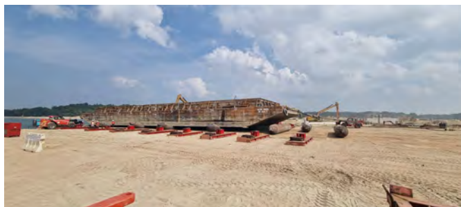
Each barge was pulled out of the water by winches with airbags underneath.
