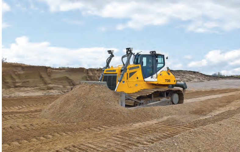
ABOVE: All Generation 8 dozers feature a hydrostatic travel drive that ensures smooth, precise movement, maximising efficiency across all operating conditions. Here is the PR 736 G8 model.
