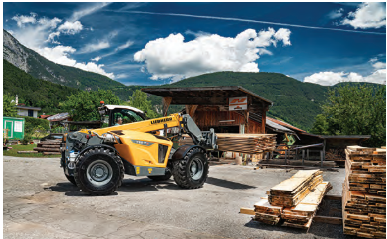
BELOW: The hydrostatic drive system, a defining feature of all Liebherr telehandlers, continues to ensure exceptional manoeuvrability, minimal wear and excellent power transmission.
